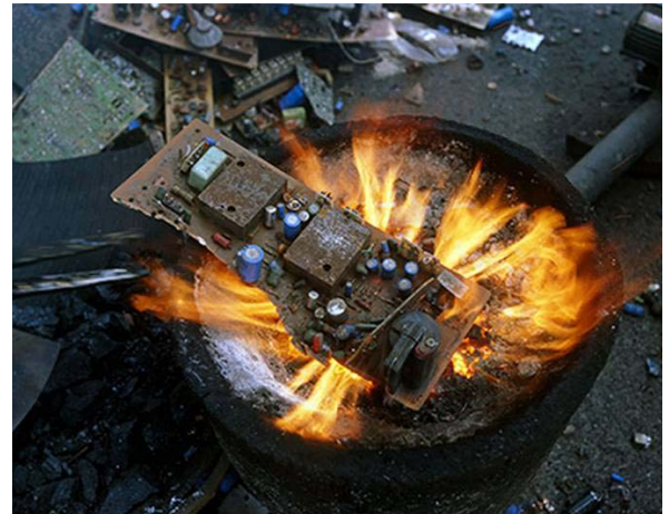
Circuit board being cooked to melt solder in Taizhou, China 2007. China illegally imports electronic waste from the US and other developed countries, where it is processed in backyard operations like this one. Photo © 2007 Stuart Isett/www.isett.com
